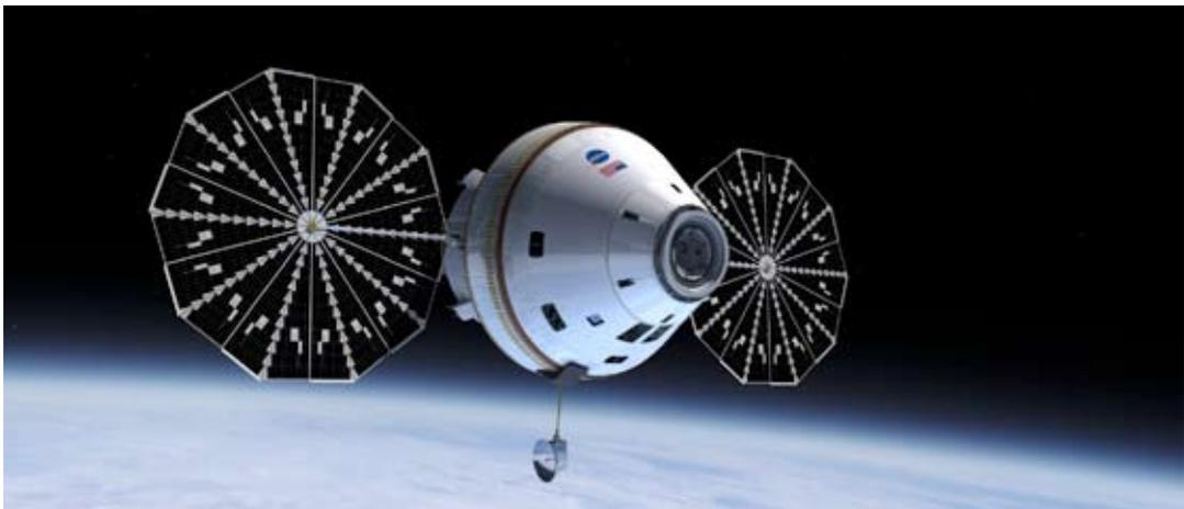
**Figure 3:** Orion vehicle in low earth orbit with solar arrays deployed.
