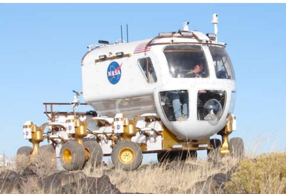
**Figure 10:** The enclosed rover concept being tested in the Arizona desert. The rover shares the ~~shared~~ chassis of the “chariot” concept.
