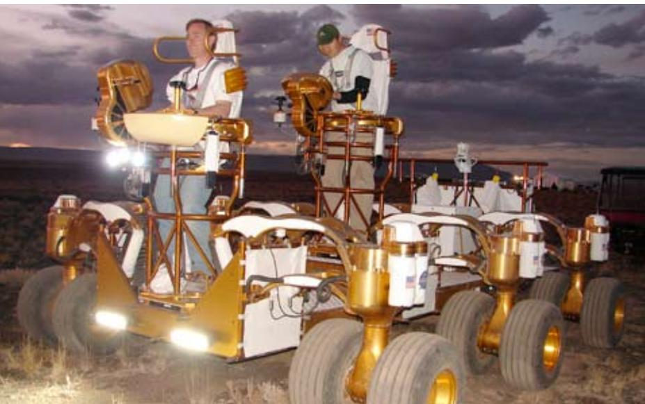
**Figure 9:** An evening test run of the NASA-prototyped “chariot” concept in the Arizona desert.
