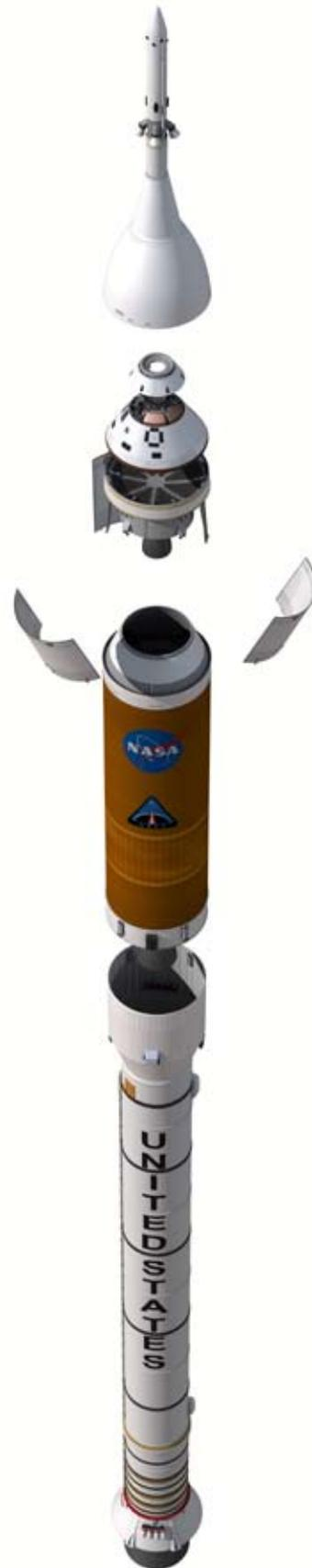
**Figure 6:** Exploded view of the Ares I vehicle with Orion in its position at launch. Image courtesy NASA/John Frassanito & Associates
